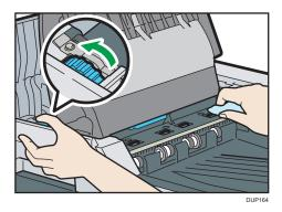
• Output rollers (4 rollers on the lower side)
