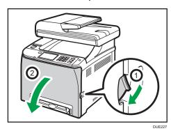
2. Lower the fusing unit lever, and pull out the jammed paper carefully.
