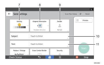
No. Icon Description Press to specify the density to scan the original. 7 You can also specify the density by touching the 💂 icon and dragging it right or left. Press to select the orientation of the original. 8 €R 2 Press to specify the sender. Press to enter the subject of the e-mail. 10 11 Text Press to enter the main text of the e-mail.
