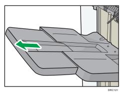
4. Attach the thin paper support tray by setting its protrusions onto the back fence of the finisher shift tray.
