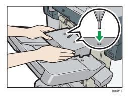
\*1 The back of the Z-fold support tray is embossed with "5".
