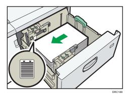
While pressing the release button of the end fence, align the end fence gently against the paper you loaded.
