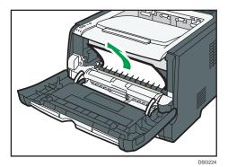
14. Slide the print cartridge in horizontally. When the cartridge can go no further, raise it slightly and push it fully in. Then push down on the cartridge until it clicks into place.
