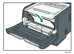
6. Slide the print cartridge in horizontally. When the cartridge can go no further, raise it slightly and push it fully in. Then push down on the cartridge until it clicks into place.
