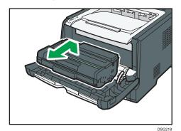
• Do not shake the removed print cartridge. Doing so can cause remaining toner to leak.
