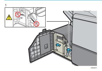
Keep your hands clear of the internal cutting blade when you are removing jammed paper. Not doing so risks injury to your fingers from the cutting blade.
