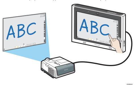
The machine cannot be connected to an analog input terminal such the VGA input of a projector.
