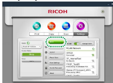
**6. If the Wi-Fi setting is disabled, toggle the [WLAN] switch to enable the Wi-Fi function.**
