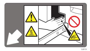
Do not touch the parts a label indicates. The inside of the machine could be very hot. Caution should be taken when removing misfed paper.
