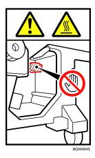
Do not touch the parts a label indicates. The inside of the Multi-Folding Unit could be very hot. Caution should be taken when removing misfed paper.
