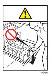
Do not press the internal unit that has been pulled out. Pressing the internal unit may cause it to fall down. 5
