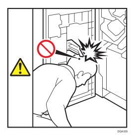
Be careful of the protruding parts of the front cover when replacing the cartridge in the saddle stitch unit or clearing a paper jam from the saddle stitch unit.
