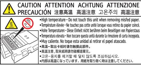
Do not touch the parts a label indicates. The inside of the machine could be very hot. Caution should be taken when removing misfed paper.
