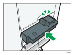
• Do not open the ink collector unit cover other than when replacing the ink collector unit. Doing so may result in misfeeds.
