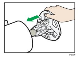
14. Insert the spool into the left flange, and then lower the lock lever on the left flange.
