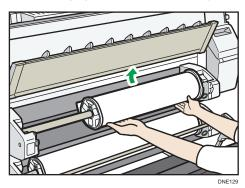
When you insert the paper between the guides, it is clamped internally.
