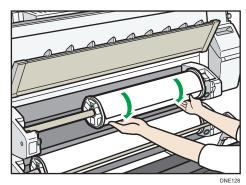
17. Rotate the paper roll so that the edge of the paper goes above the lower guides.
