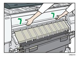
5. Pull up the paper holding lever on the right of the machine.
