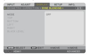
This adjusts the edges (boundaries) of the projection screen when projecting high resolution videos using a combination of several projectors in the up, down, left and right positions.
