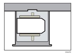
If you are copying or printing onto side-opening envelopes in the  $\square$  orientation, flaps must be at the right side of the wide LCT or multi bypass tray (Tray 7). If you are copying or printing in the  $\square$  orientation, flaps must be at the bottom side of the three-tray wide LCT or multi bypass tray (Tray 7). Be sure to load the envelopes with print side face up.
