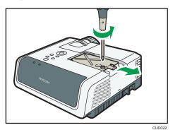
3. Loosen the two screws on the left side of the lamp unit.
