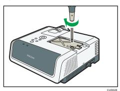
10. Put the outer lamp cover on the projector, and then slide it to the left.
