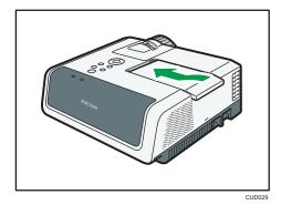
Make sure the projections on the left edge of the outer lamp cover are inserted into the holes on the projector properly.
