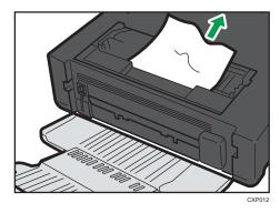
6. If it is difficult to remove the jammed paper out of the main unit, remove the jammed paper from the output tray side.
