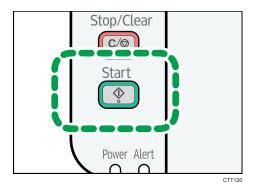
5. Within 30 seconds, place the original back side down with the top to the rear of the machine on the exposure glass, and then press the [Start] key.
