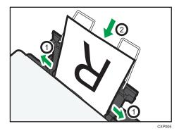
6. Adjust the paper guide on both sides to fit the paper width.
