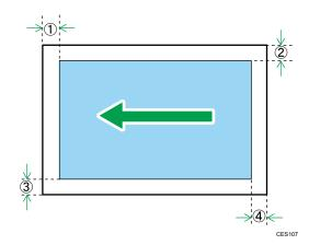
Margins when using exposure glass
