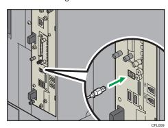
When connecting the USB interface cable to the USB2.0 (Type B) port on the Gigabit Ethernet board
