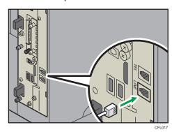
2. If using an external telephone, connect the telephone to the external telephone connector (TEL).
