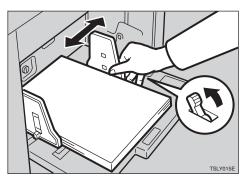
Adjust the side plates of the paper delivery tray to match the new paper size.
