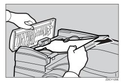
If you are unable to remove the misfed original in Step **2**, lift the document feeder.
