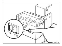
Press the manual cut button to trim off the leading edge of the tape.
