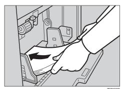
Make sure that the paper feed side plates touch the paper lightly. Shift the lock lever back to its original position.
