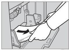
Shift the paper feed side plate lock lever forward. Adjust the paper feed side plates to match the paper size.
