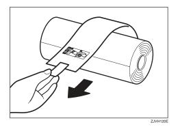
A Remove the used master roll and pull out both spools. Then, insert both spools into a new master roll.
