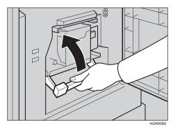
Pull out the drum unit by its handle.
