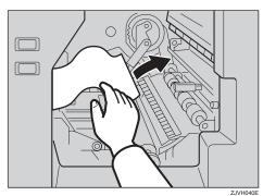
Insert the drum unit until it locks in position, and then lower the drum unit lock lever.
