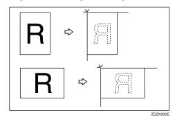
The first 5mm, 0.2", of the leading edge cannot be printed. When using the optional document feeder, the first 5mm, 0.2", of the leading edge as well as the last 2mm, 0.08", of the trailing edge cannot be printed.
