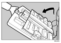
2 Lift the paper delivery side plates and adjust them to match the paper size.
