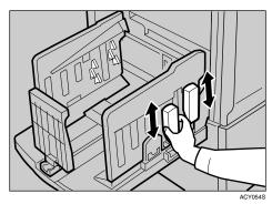
Adjust the paper alignment wings and chocks according to paper size and thickness, as follows:
