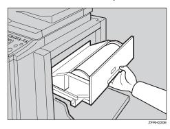
**2** Open the master feeding cover, and then remove the misfed master inside.
