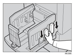
Move the paper delivery end plate until its handle is flush with the end of the tray.
