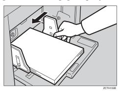
After you have finished printing, return the feed roller pressure lever to the Standard paper position.
