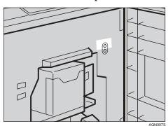
2 Lift to unlock the drum unit lock lever.
