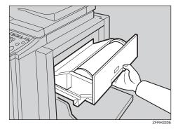
**2** Press the release button to open the master feeding cover.
