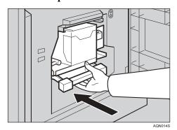
**1** Lower the drum unit lock lever.
