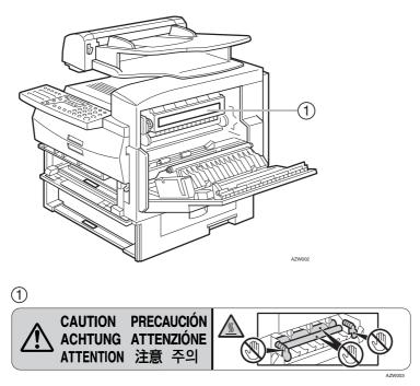
High temperature. Be careful of hot parts when clearing paper
