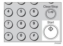
The machine calls the destination. While it is dialing, the number or name which is programmed as the Own Name or Own Fax Number in the machine of the other party is shown on the display. When connected, the machine starts scanning the original.
