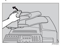
While pushing the release button, lift the ADF unit.
