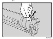
Insert the toner cartridge and make sure it locks securely into place.
