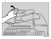
While pushing the release button, lift the ADF unit.
