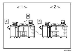
When machine <1> has finished with Original A, it begins copying Original C.
