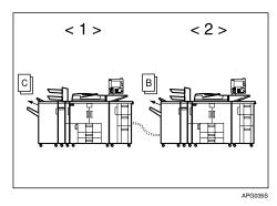
When machine <2> has finished with Original B, it also begins copying Original C.
