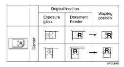
This table shows the stapling positions, not the orientation of delivery.
