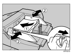
2 Attach the back fence to the end fence, and then set the end fence.
