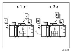
When machine <1> has finished with Original A, it begins copying Original C. If machine <1> finishes copying it allotment of Original C before machine <2> finishes with Original B, machine <1> will take over to copy the remainder of Original C.
