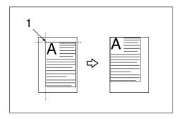
① Point from which the machine begins scanning
