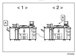
Machine <2> begins copying Original B. Machine <1> also starts copying Original B when it has finished with Original A.
