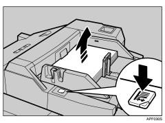
The green lamp of the elevator switch is blinking while the original table is going up and down, and keeps lit when it stops.
