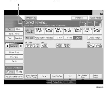
1. Sub-machine status appears on the second line of main machine's display.
