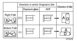
The above table shows Z-folding positions. The orientation of the paper does not indicate direction of delivery.
