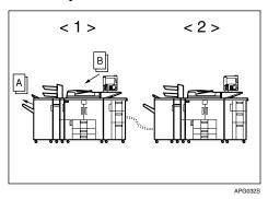
When machine <1> has finished with Original A, Connect Copy is activated and both machines begin copying Original B.
