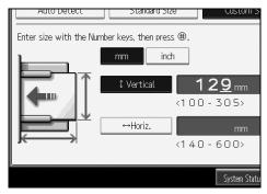
Specify a horizontal size from 140 mm (5.5") to 600 mm (23.6"). You cannot enter a size smaller than 140 mm or larger than 600 mm.
