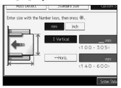
Specify a vertical size from 100 mm (4.0") to 305 mm (12.0"). You cannot enter a size smaller than 100 mm or larger than 305 mm.
