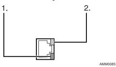
Indicator (green)Remains green when the machine is properly connected to the network.
