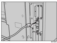
**1** Connect the other end of the Ethernet cable to a network connection device such as a hub.
