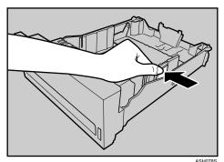
Pinch the clip on the end paper guide and align the arrow with the paper size.
