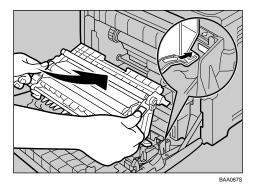
Slide the transfer unit along the guide rails into the machine. When it stops, push on the green PUSH mark until it clicks into place.
