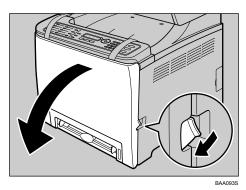
8 Lower the blue fusing unit levers.
