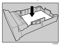
Lift and slide the tray, then push it all the way in. Push the tray firmly to avoid a paper jam.
