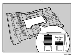
Carefully slide the paper tray back in until it stops. To avoid paper jams, make sure the tray is securely inserted.
