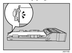
If there is a gap between the paper and the front end paper guide, as in the example below, the paper might not feed in correctly.
