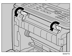
**5** Using a coin, turn both gray knobs on the fusing unit 90 degrees counterclockwise (until the slots are horizontally aligned with the ☆ marking shown in the illustration below).
