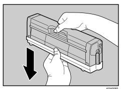
**6** Check that the toner color and location correspond, and carefully insert the print cartridge vertically.
