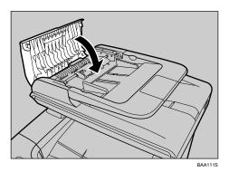
**7** Pull the opening lever on the front cover, and then carefully lower the front cover.
