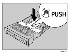
Reload the removed paper into the tray, and then push the tray carefully into the machine until it clicks into place.
