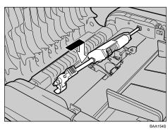
2 Lower the green lever to lock the paper feed roller.
