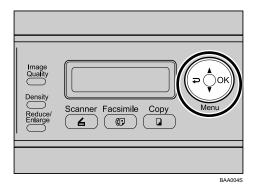
Press the [▲][▼] keys to select [Scan Settings], and then press the [OK] key.
