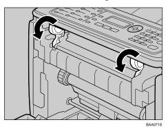
**1** Using a coin, turn both gray knobs on the fusing unit 90 degrees clockwise (until the slots are vertically aligned with the ○ marking shown in the illustration below).
