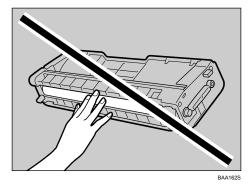
☐ When removing print cartridges, be careful not to touch the Laser Scanning Unit on the underside of the upper cover (the white area in the illustration below).
