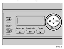
Press the [▲][▼] keys to select [Copy Settings], and then press the [OK] key.
