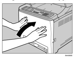
Pull up the top cover open lever, and then open the top cover carefully. Make sure that the exposure glass cover or ADF is closed.
