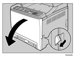
**3** Lower the blue fusing unit lever.
