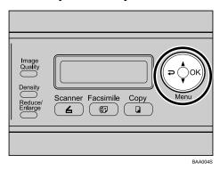
Press the [▲][▼] keys to select [Fax Settings], and then press the [OK] key.
