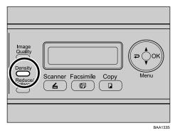
Press the [Density] key or [▲][▼] keys to select the desired density level, and then press the [OK] key.
