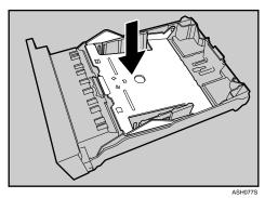
Pinch the clips on the side paper guide, and then adjust the guide to the paper size.
