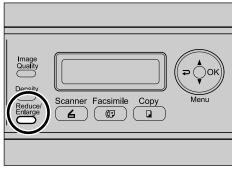
Press the [Reduce/Enlarge] key or [▲][▼] keys to select the size of the original, and then press the [OK] key.
