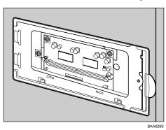
To install the memory unit, align the notch of the unit with the protruding part of the slot, and then carefully push in the unit at an angle.
