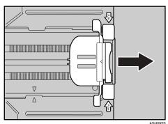
After extension, make sure the arrows on the extender and tray are aligned.
