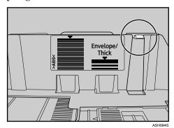
Check there are no gaps between the paper and the paper guides; both side and front end paper guides.
