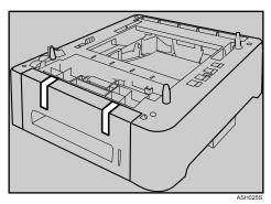
**1** Lift using the inset grips on both sides of the machine.
