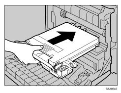
To prevent the waste toner bottle touching the intermediate transfer unit (the white area in the illustration below), do not lift the bottle while inserting it.
