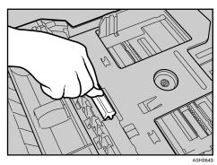
Wipe the rubber part of the roller with a soft damp cloth. After that, wipe it with a dry cloth to remove the moisture.
