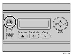
Press the [Image Quality] key or [▲][▼] keys to select the desired resolution setting, and then press the [OK] key.
