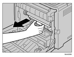
Pull the waste toner bottle halfway out, grab the bottle firmly, and then pull it straight out.
