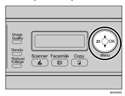
Press the [▲][▼] keys to select [PDL Settings], and then press the [OK] key.
