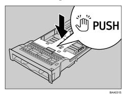
Pinch the clip on the side paper guide, and then adjust the guides to the envelope.
