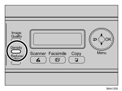
Press the [Density] key or [▲][▼] keys to select the desired density level, and then press the [OK] key.
