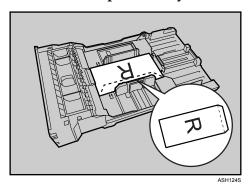
Make sure envelopes are not stacked higher than the upper limit (lower line) mark inside the tray.
