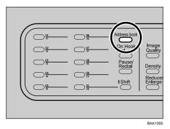
2 Enter the registered number (1-50) of the Speed Dial entry using the number keys, and then press the [OK] key.
