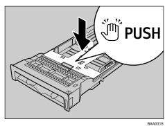
Pinch the extender in the "PUSH" direction, and then pull out the extender until it stops (you will hear a click).
