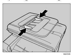
Place the aligned originals face up in the ADF. The last page should be on the bottom.
