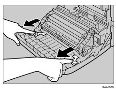
Holding the green tabs on both ends of the transfer unit, tilt it backwards then lift it up.
