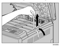
**E** Lift out a print cartridge and shake it from side to side five or six times.
