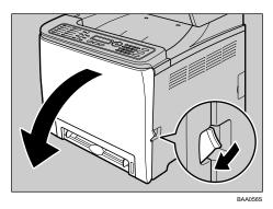
2 Lower the blue fusing unit lever, and pull out the jammed paper carefully.
