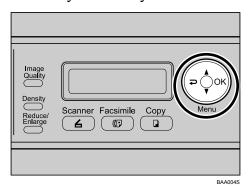
Press the [▲][▼] keys to select [Copy Settings], and then press the [OK] key.
