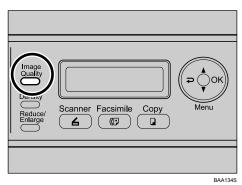
Press the [Image Quality] key or [▲][▼] keys to select the desired document type, and then press the [OK] key.
