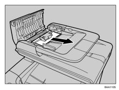
If you cannot pull out the jammed original easily, unlock the paper feed roller by raising the green lever.
