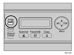
Press the [Image Quality] key or [▲][▼] keys to select the desired resolution, and then press the [OK] key.
