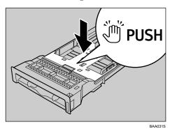
Pinch the clip on the side paper guide and slide it to match the standard size.
