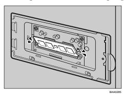
**1** Attach the inner cover, and then fasten the screw.
