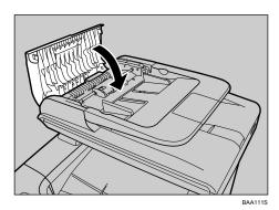
Lift the ADF, and if there is original remaining in the ADF, gently pull the jammed original to remove it.
