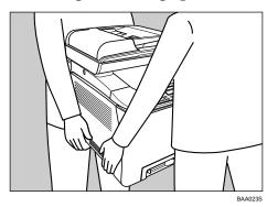
There are three upright pins on the optional paper feed unit. Align them with the holes on the underside of the machine, and then carefully lower the machine onto them.
