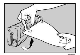
Check the toner color and corresponding location, and then carefully insert the print cartridge vertically.
