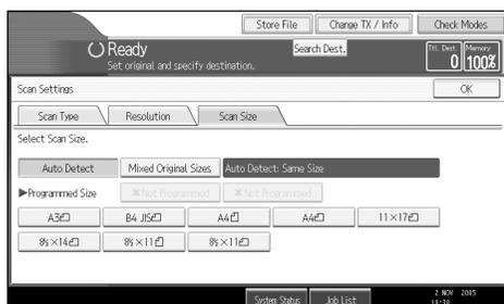
8<sup>1</sup>/<sub>2</sub>"×11" indicates LT. 8<sup>1</sup>/<sub>2</sub>"×14" indicates LG. 11"×17" indicates DLT.
