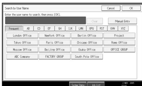
To search by directly entering a user name, press [**Manual Entry**], and then enter the user name. Partial matching is used when searching for a user name.
