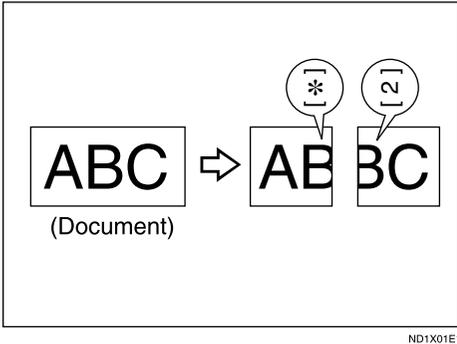
For example, this function splits the document if the document length is 20 mm (0.79") or longer than the paper used. The document is reduced if it is less than 20 mm (0.79"). When a document is split, an asterisk (✱) is inserted at the split position and about 10 mm (0.39") of the split area is duplicated on the top of the second sheet.
