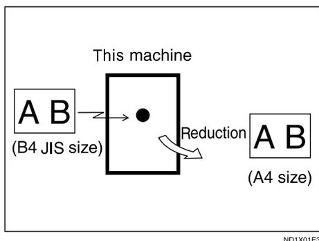
If you turn this function on, the machine reduces the width and length of the received image so that it will fit on one page. If A4 paper is loaded and a document of B4 JIS size is received, the machine will reduce the document to a single A4 sheet.
