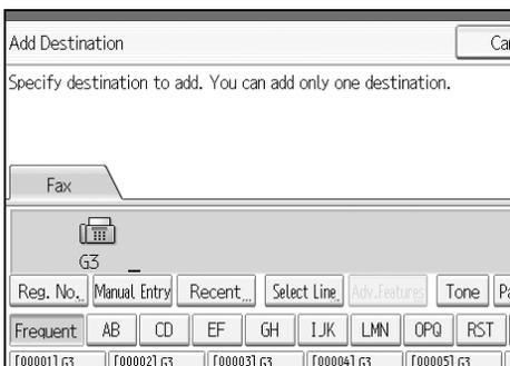
When the file has some Internet Fax destinations, you can switch the transmission type between fax/IP-Fax and Internet Fax by pressing **[Fax]** or **[Internet Fax]**.
