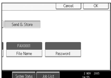
**2** Enter a password using the number keys, and then press [OK].
