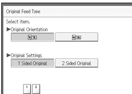
Make sure that the specified original orientation matches the orientation of originals loaded in the ADF.
