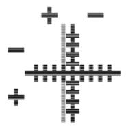
Fold the test pattern sheet in half widthwise, and then check the adjustment value for the [Feed Direction]
