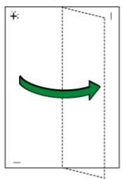
9. The optimal adjustment value is the difference between the single vertical line and the cross's vertical line that you can see when the folded paper is held up to light. When the difference is one calibration mark in the "+" direction, the optimal adjustment value for the [Read Direction] is "+1.0".
