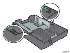
6. Load paper print side down, and then adjust the paper guide to the paper size.
