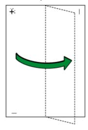
10. The optimal adjustment value is the difference between the single vertical line and the cross's vertical line that you can see when the folded paper is held up to light. When the difference is one calibration mark in the "+" direction, the optimal adjustment value for the [Printing direction:] is "+1.0".
