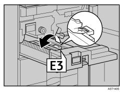
13. Remove the paper being careful not to touch the area around the lever E3.
