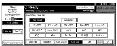
Specify Original Size (X1 and Y1) using the number keys, and then press the [#] key.
