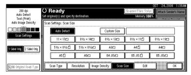
Specify Original Size (X1 and Y1) using the number keys, and then press the [#] key.
