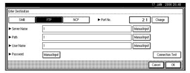
A connection test is performed to check whether the specified folder exists.
