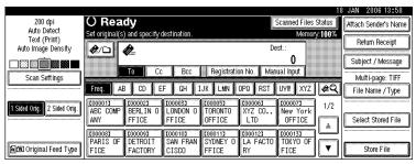
2 Using the number keys, enter the five-digit registration number assigned to the required destination folder.
