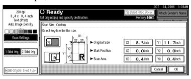
Specify Start Position (X2 and Y2) using the number keys, and then press the [#] key.
