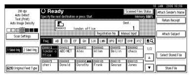
2 Using the number keys, enter the three-digit registration number assigned to the required destination folder.
