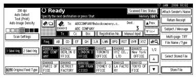
2 Using the number keys, enter the five-digit registration number assigned to the required destination folder.
