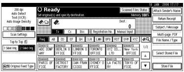
**2** Select [2 Sided Orig: T to T] or [2 Sided Orig: T to B] according to the binding orientation of the original.
