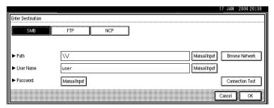
A connection test is performed to check whether the specified shared folder exists.
