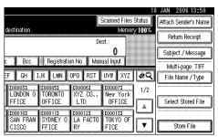
Up to 5 transmission or delivery results are displayed at the same time. Press [▲Prev.] or [▼Next] to switch between results.
