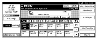
The selected destination is highlighted and also is displayed in the destination field at the top of the screen.
