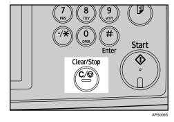
Pressing the [Clear/Stop] key deletes by single digits the fax number or IP-Fax address. The Internet Fax address can be entirely deleted at once by pressing the [Clear/Stop] key.
