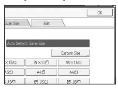
Specify Original Size (X1 and Y1) using the number keys, and then press [#]. For example, set X1 to 17.0 inch and Y1 to 8.0 inch.
