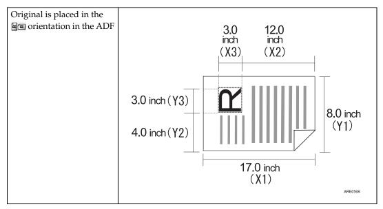
Examples 1 and 2 (above) explain the procedure for scanning the "R" area of the original.
