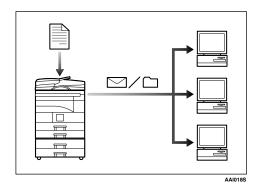
• You can send scan files to a specified destination using e-mail (Sending scan file by e-mail). See Scanner Reference.  With ScanRouter V2 Professional\*/Lite, you can save scan files in specified destinations on network computers (Using the network delivery scanner function). See Scanner Reference.
