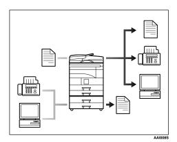
This machine provides copier, facsimile\*, printer\*, and scanner\* functions.
