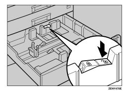
While pressing the release lever, adjust the side fences.
