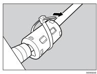
Fit the other tie wrap snugly around the end of the ferrite core to prevent the core moving along the cable.
