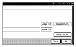
A connection test is performed to check whether the specified shared folder exists.
