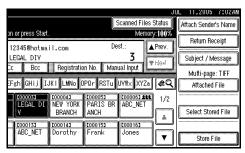
2 Enter the five digit registration number that has been assigned to a destination folder using the number keys.
