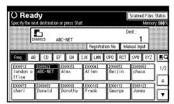
The selected destination is highlighted and also is displayed in the destination field at the top of the screen.
