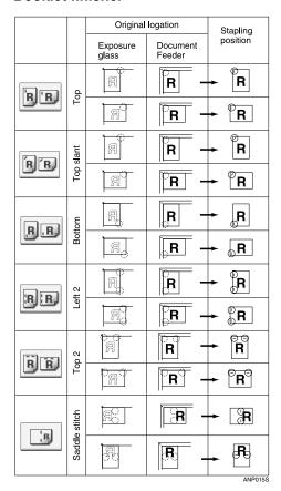
This table shows the stapling positions, not the orientation of delivery. Not available for vertical Left 2 and horizontal Top 2 for A3 or B4 JIS size paper.
