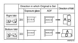
The above table shows Z-folding positions. The orientation of the paper does not indicate direction of delivery.
