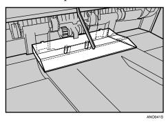
Close the front cover of the finisher. The Z-fold support tray is lowered to complete the installation.
