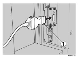
To make the connection, use the conversion connector (1) supplied with the optional IEEE 1284 interface board.
