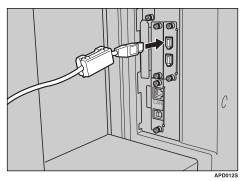
For IEEE 1394 (SCSI print) connection, plug the other end of the cable into the interface connector on the host computer.
