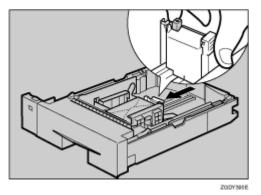
Lift the front of the tray, and then slide it carefully into the printer until it stops.
