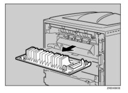
Push down the lever on right side of the duplex unit (1) and pull it out until it stops (2).
