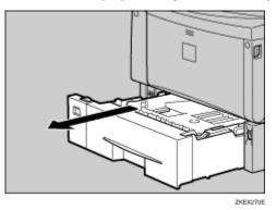
Lift the front side of the tray, and then pull it out of the printer.
