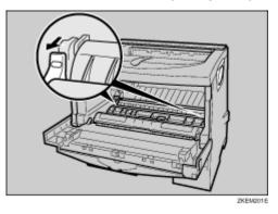
• Hold the green parts of the roller on both sides, and remove the roller from the printer as shown in the illustration.
