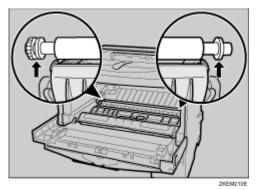
Insert the new transfer roller on the socket with the gear of the roller positioned on the left.
