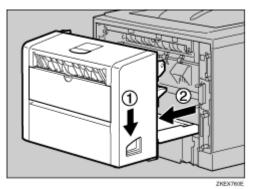
Push the under board levers (1) and pull the duplex unit out of the printer (2).
