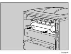
**5** Pull out the pins on both sides of the new fusing unit.
