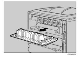
**1** Lift the lock levers of the fusing unit as shown in the illustration.
