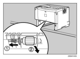
Wipe the rubber part of the roller with a soft damp cloth. Then, wipe it with a dry cloth to remove the water.
