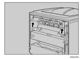
Pull the fusing unit out.
