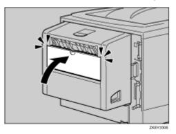
Lift the lever (1), open the cover of the duplex unit (2).
