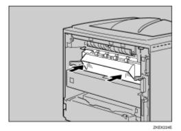
Push the lock levers of the fusing unit down until it clicks.
