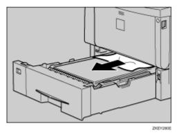
**2** Carefully slide the paper tray into the printer until it stops.
