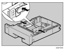
Pinch the rear guide, and then slide it along the edge of the envelope stack.
