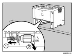
While sliding the green lock lever to the left (1), set the new roller (2). Then, return the green lock lever to its original position (3).
