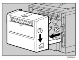
**2** Lift the guide board inside the duplex unit, and remove the misfed paper.
