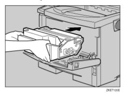
**5** Lower the toner cartridge when it makes contact in the back.
