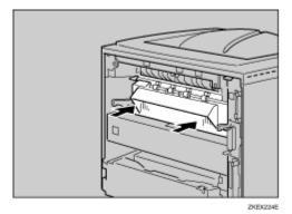
$I\!\!I$  Push the lock levers of the fusing unit down until it clicks.
