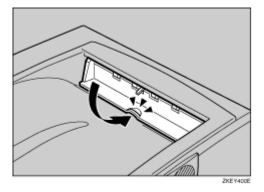
Open the front cover by pushing the front cover release button.
