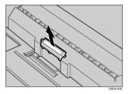
**1** Insert the new friction pad in the paper tray.
