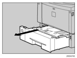
**2** Lift the front side of the tray, and then pull it out of the printer.
