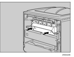
**2** Push the lock levers of the fusing unit down until it clicks.
