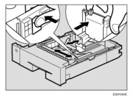
Push the bottom plate down until it locks into place.
