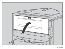
${f E}$  Push in the duplex unit along the rails in the back of the printer.
