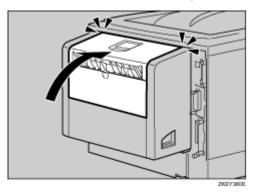
Removing misfed paper inside the duplex unit
