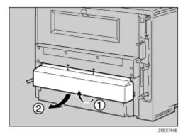
Lift the front side of the tray, and then place it into the printer. Carefully slide it into the printer until it stops.
