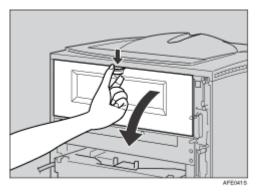
**2** Remove the rear cover in a horizontal direction.
