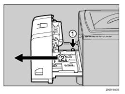
**1** Lift the lock levers of the fusing unit as shown in the illustration.
