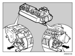
**6** Replace the new fusing unit into the printer.
