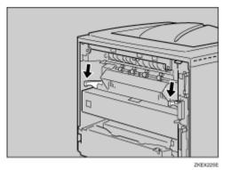
B Push in the duplex unit along the rails in the back of the printer.
