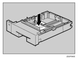
**E** Load envelopes into the envelope feeder unit, with the print side down and the flap on the left as shown in the illustration.
