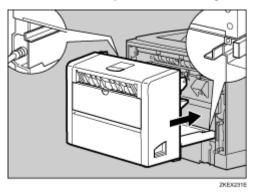
Securely push the duplex unit into the printer.
