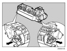
Beplace the new fusing unit into the printer.
